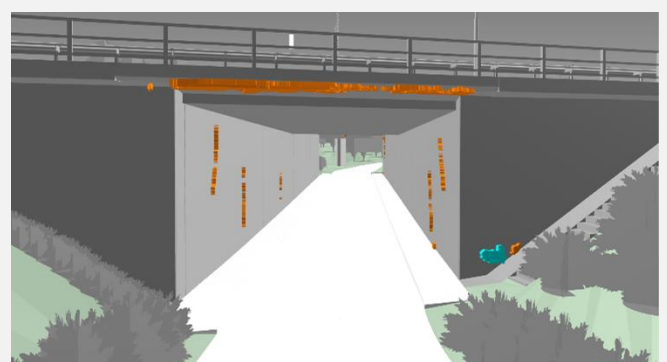
BIM Integration of the AI detected damages
