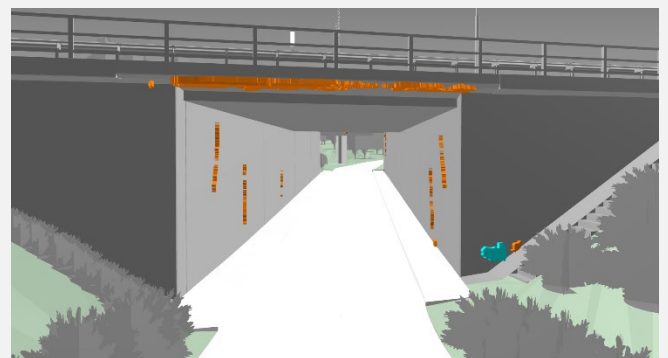
BIM integration of the AI detected damages
